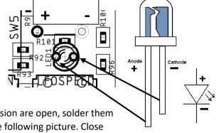
11. If all jumpers SJ1...SJ7 in your DIY kit version are open, solder them on Board 1 and Board 2 according to the following picture. Close the jumper at the point indicated by the arrow.
