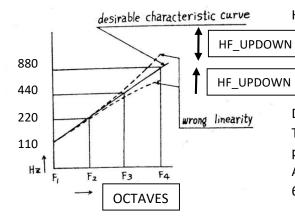
HF\_UPDOWN, HF\_UP trimmers allow you to bend the 1V/OCT curve and achieve a more precise desired oscillator setting
